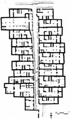
Street Layout in Jaisalmer, Rajasthan: The north-south-running street assures that only a narrow front of each house is exposed to the most critical summer sun that comes mainly from the east and west. Tall houses facing each other across the narrow street also provide a mutual shield. ( Paradigms of Indian Architecture by G. H. R. Tillotson 1998, 162.)
